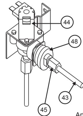
**NOTICE** A brass compression nut [45], a brass sleeve, a plastic sleeve [46], and a brass insert [47] are supplied and attached to the rear of the refrigerator (See Art01604).
