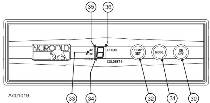
The TEMP SET button [32] controls the temperature adjustment of the freezer and the fresh food compartment. The temperature adjustment that you select does not change if the mode of operation of the refrigerator changes.
