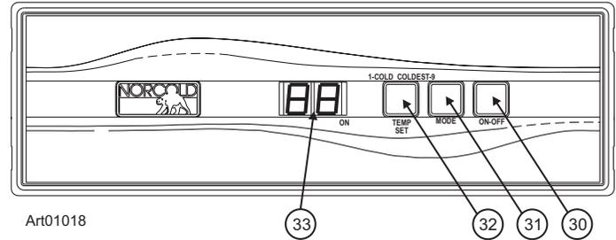
The ON / OFF button [30] starts and shuts down the refrigerator:
