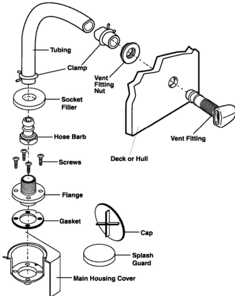
1. Remove Cap and Splash Guard from Electra-Magic Main Housing Cover on the side desired for the Vent Kit installation.
